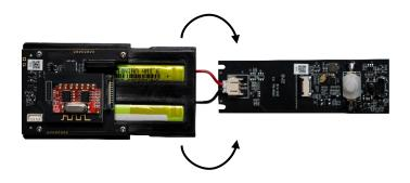
6. Remove the green battery pack from the holder and disconnect it from the circuit board at the white connector.
