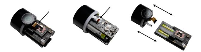
5. Now separate the two boards that are now visible and plugged into each other.
